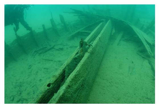
Figure 7. Centerboard trunk and centerboard. Looking forward on the starboard side.
