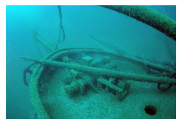
Figure 14. Windlass, bowsprit, and jibboom viewed from aft. The yard is visible lying across the windlass and the forecastle companionway.
