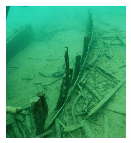
Figure 8. Port chainplate attached to frame, looking aft.
