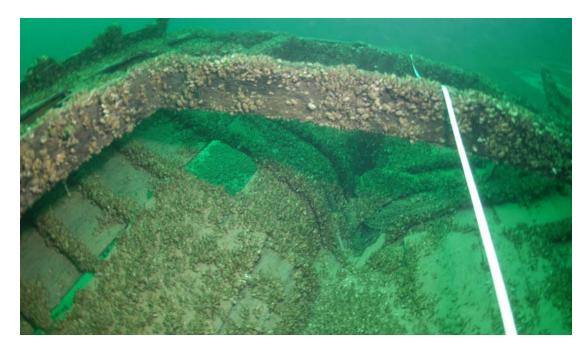
Figure 34. Frames and ceiling planks visible through cabin opening.
