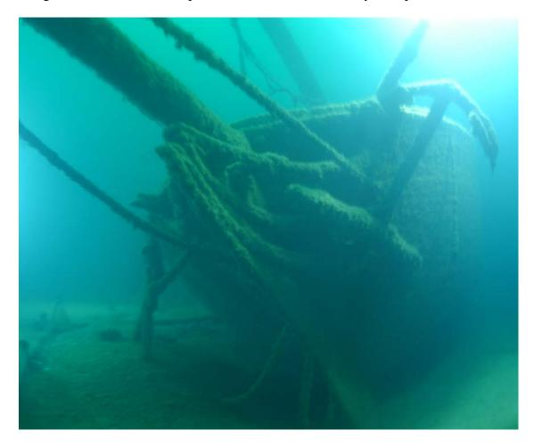
Figure 13. View of the ornate bow from the port side. Note the empty ledge where the fiddle- or billethead once stood.
