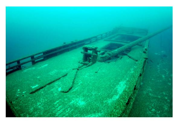
Figure 26. Centerboard winch, looking aft. The missing deck plank over the centerboard trunk is visible, as is the loose plank with chain attached.
