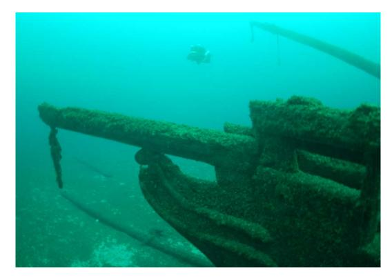
Figure 41. A rare billethead remains intact on the *Northerner*'s bow knee.
