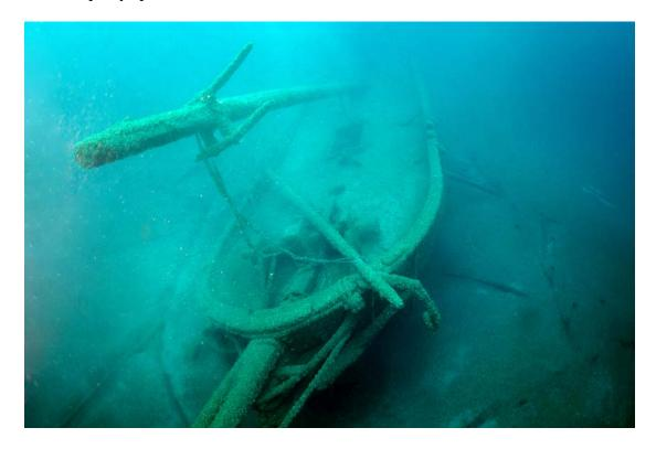
Figure 17. The mainmast has toppled forward with trestle trees and tops intact. Looking aft from above the bowsprit. Note tangle of fish net on either side of the hull.
