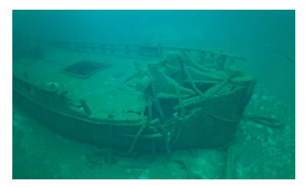
Figure 23. Damage on starboard side bow. Bowsprit and anchor fluke are visible on the lakebed near the stem.
