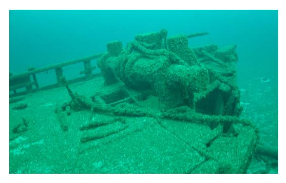
Figure 24. Windlass viewed from starboard aft. Forecastle hatch is visible beneath windlass, and the bilge pump and foremast aft of that.
