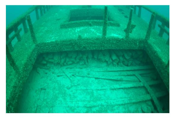
Figure 47. The cabin opening, looking forward. Frames for the cabin bulkheads are extant, and the wood cargo is visible, neatly stacked in the hold.
