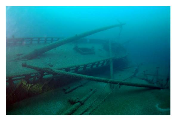
Figure 19. Many of the vessel's spars lie off the starboard side. The fore yard lies across the windlass, and a boom lies across the starboard rail. A topmast lies underneath the boom, with a gaff lying nearer the hull. A smaller yard is visible lying off the starboard bow. Most of the spars are tangled in fish net.
