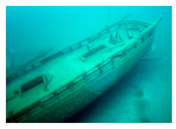
Figure 15. Stern deck arrangement with below-deck cabin. Note missing wheel.
