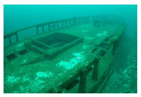
Figure 45. The forward cargo hatch, looking aft from the port side. Gaps in the bulwark stanchions are visible on either side of the hatch. The starboard gap on the aft cargo hatch is also visible.
