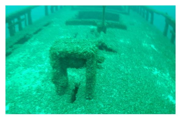
The ends of the shafts are square, requiring a winch handle to be installed in order to raise or lower the centerboard.
